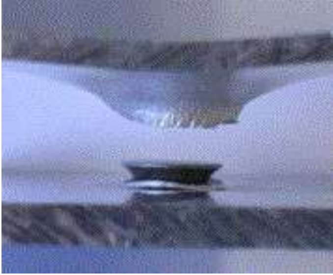
Figure 3. Typical failure modes of SPR joint: rivet head pull-out.
