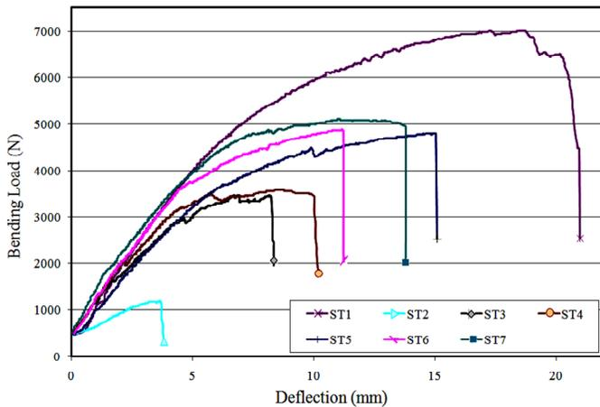
**Figure 16.** Synthesis of failure load values obtained from experimental results.
