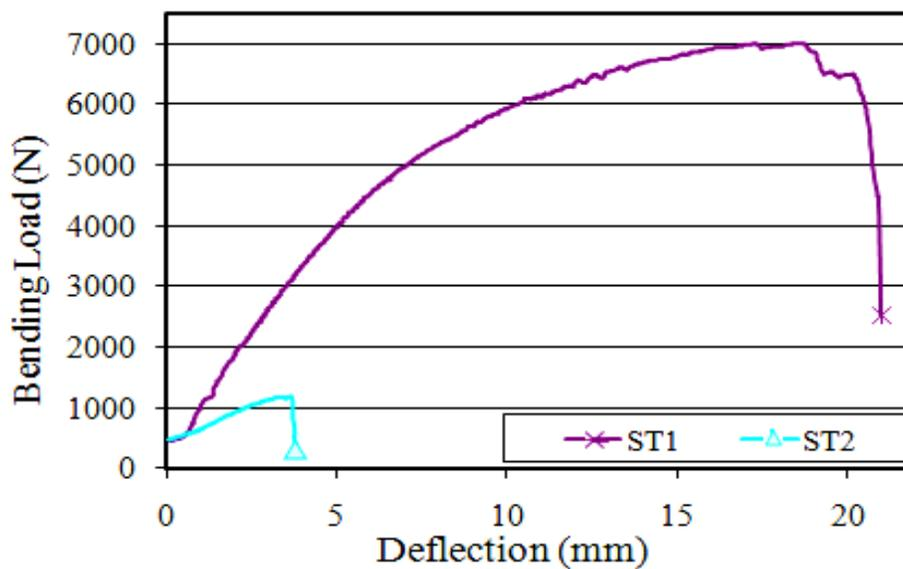
Figure 8. Load-deflection behaviours of massive and connection with un-strengthened timber beams.
