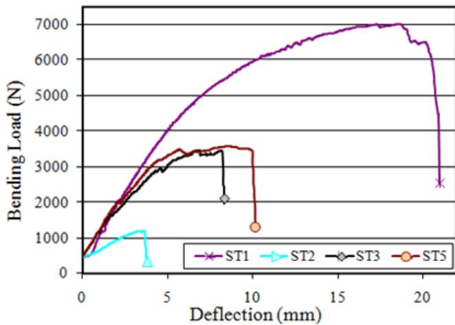
**Figure 11.** Load–deflection behaviours of massive, connection without reinforcement and connection with a GFRP bar under and top of the timber.
