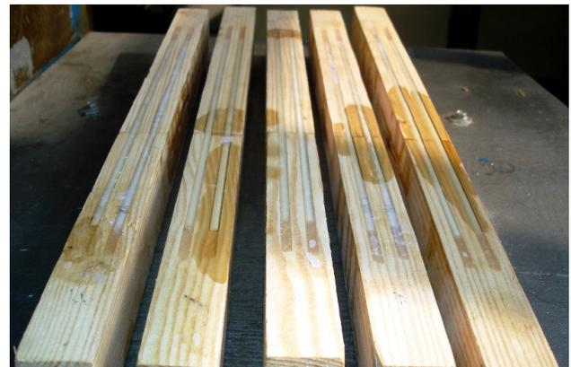
**Figure 13.** Timber connection samples with two GFRP bars.
