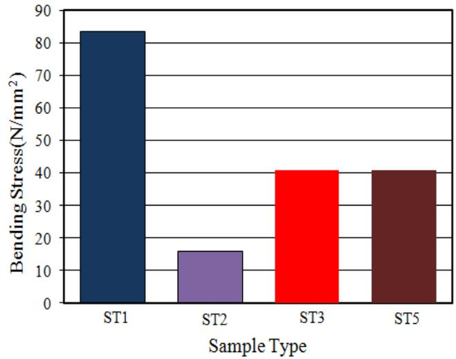
**Figure 12.** Bending strength of massive, connection without reinforcement and connection with a GFRP bar under and top of the timber.
