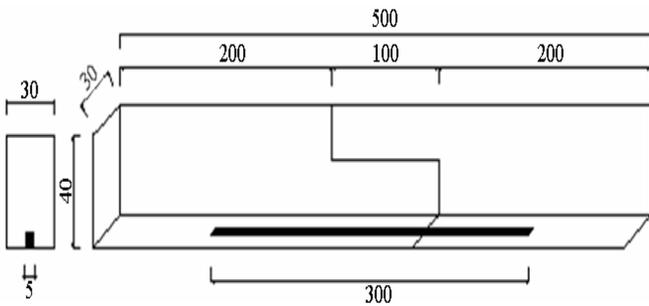
**Figure 10.** Configuration of timber connection strengthen with a GFRP bar.
