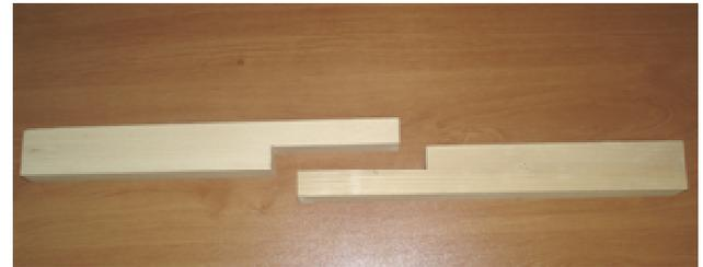
**Figure 4.** Longitudinal notched lap joint application of timber.
