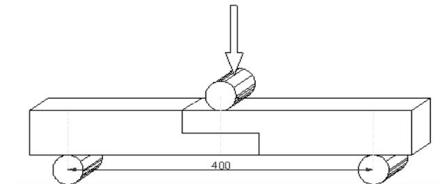
**Figure 5.** Three point bending test configurations.
