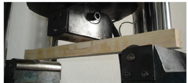
**Figure 6.** Three point bending test application.
