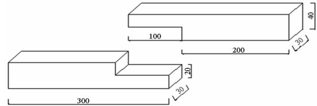
**Figure 3.** Longitudinal notched lap joint configurations.
