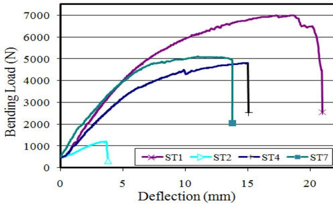
**Figure 15.** Load–deflection behaviours of massive, connection without reinforcement and connection with double GFRP bars under and single GFRP bars on the top of the samples.
