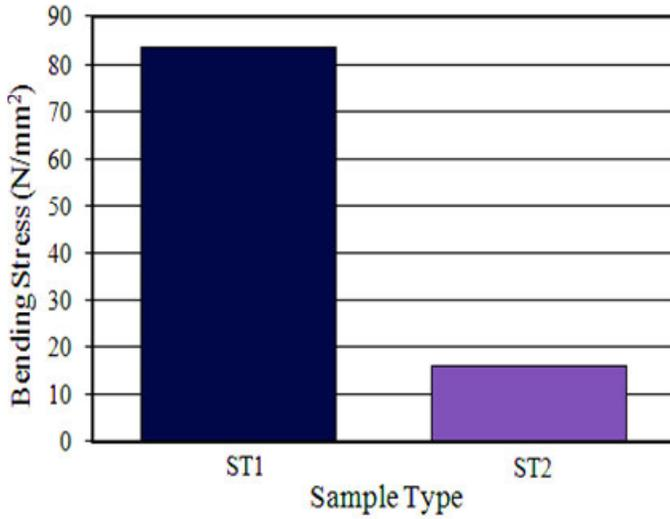
**Figure 9.** Bending strength massive and connection with un-strengthened timber beams.
