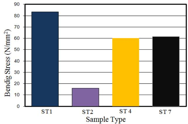
**Figure 14.** Bending strength of massive, connection without reinforcement and connection with double GFRP bars under and single GFRP bars on the top of the timber.
