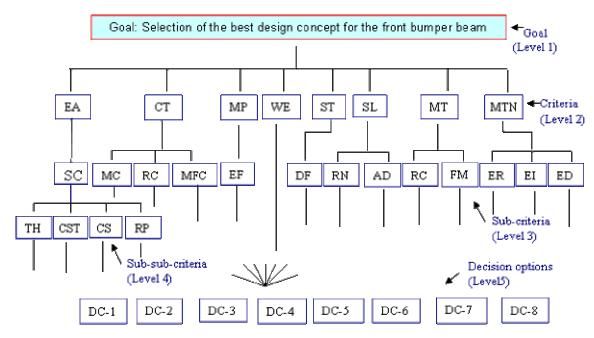
**Figure 7.** The hierarchy model (4 levels) represents the criteria and sub-criteria affecting the selection of design concepts for automotive bumper beam.
