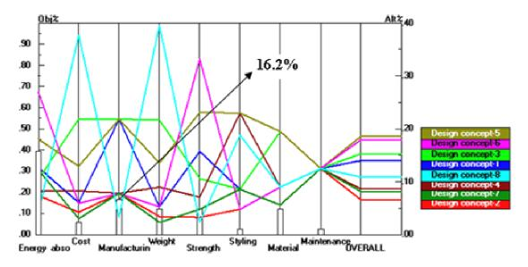
Figure 13. The sensitivity graph of the main criteria with respect to the goal when score or weight of 'manufacturing process' is increased by 10%.
