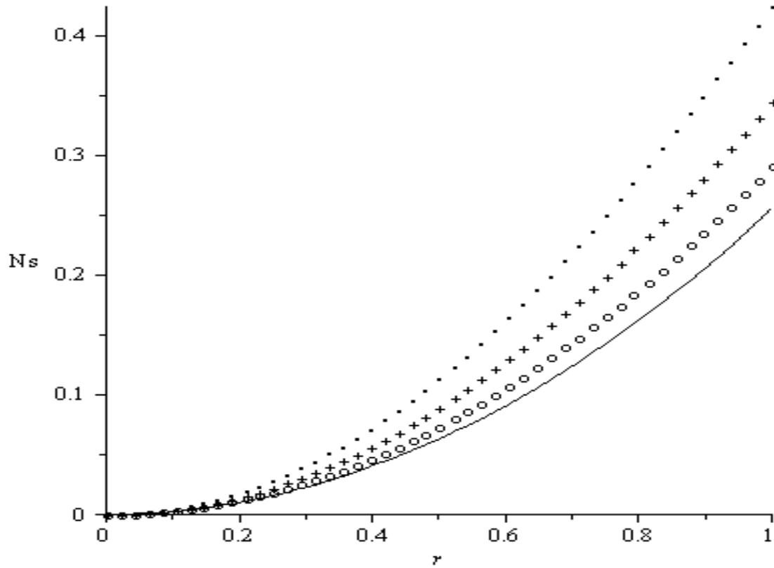
Figure 9. Entropy generation rate:  $G = 1; Br = 1; Bi = 1;$  \_\_\_\_\_  $\alpha = 0.1;$  ooooo  $\alpha = 2;$  ++++  $\alpha = 4;$  .....  $\alpha = 6.$
