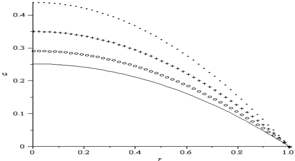
Figure 2. Velocity profile:  $G = 1$ ;  $Br = 1$ ;  $Bi = 1$ ; \_\_\_\_\_  $\alpha = 0.1$ ; oooooo  $\alpha = 2$ ; +++++  $\alpha = 4$ ; .....  $\alpha = 6$ .
