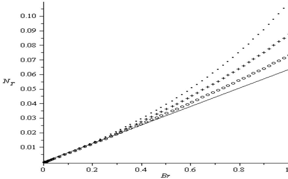
Figure 13. Total entropy generation:  $G = 1$ ;  $Bi = 1$ ; \_\_\_\_\_  $\alpha = 0.1$ ; ooooo  $\alpha = 2$ ; ++++  $\alpha = 4$ ; .....  $\alpha = 6$ .
