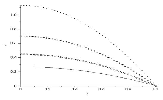
**Figure 4.** Velocity profile: Br = 1;  $\alpha = 1$ ; Bi = 1; \_\_\_\_\_G = 1; 00000G = 1.5; ++++G = 2; .....G = 2.5.
