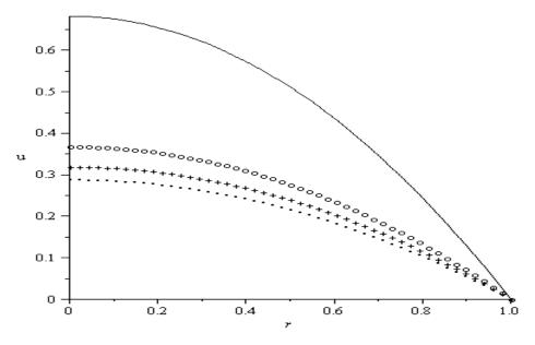
**Figure 3.** Velocity profile: G=1;  $\alpha = 1$ ; Br = 1; \_\_\_\_\_Bi = 0.1; 00000Bi = 0.2; ++++ Bi = 0.4; .....Bi = 0.5.
