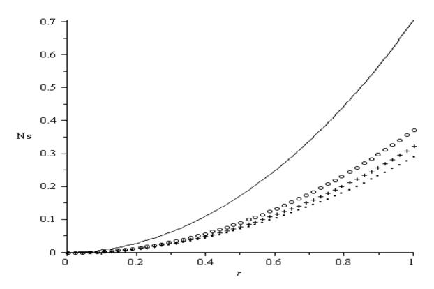
**Figure 10.** Entropy generation rate: G=1;  $\alpha = 1$ ; Br = 1; \_\_\_\_\_Bi = 0.1; oooooBi = 0.2; ++++ Bi = 0.3; .....Bi = 0.5
