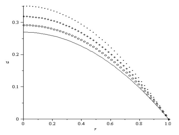
**Figure 5.** Velocity profile: G = 1;  $\alpha = 1$ ; Bi = 1; \_\_\_\_\_Br = 1; 00000Br = 2; ++++Br = 3; .....Br = 4.
