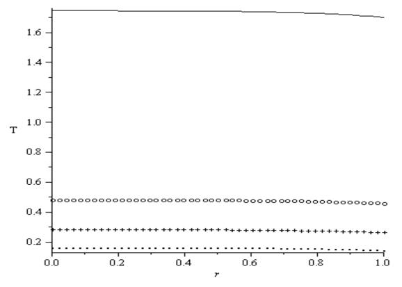
**Figure 7.** Temperature profile: G=1;  $\alpha = 1$ ; Br = 1; \_\_\_\_\_Bi = 0.1; oooooBi = 0.2; ++++ Bi = 0.3; .....Bi = 0.5
