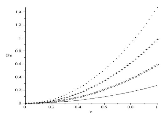
**Figure 11.** Entropy generation rate: G=1;  $\alpha = 1$ ; Bi = 1; \_\_\_\_\_Br = 1; oooooBr = 2; ++++ Br = 3; .....Br = 4.
