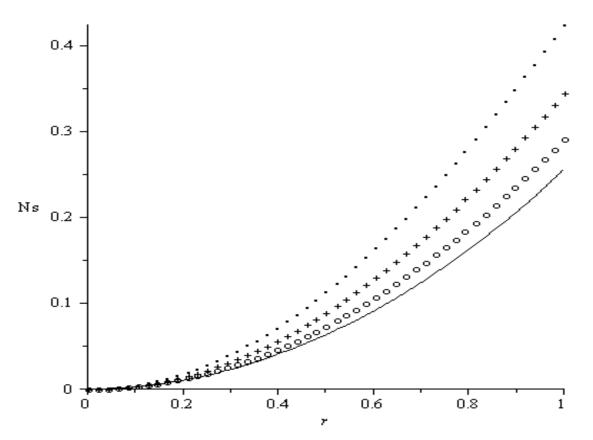
**Figure 9.** Entropy generation rate: G = 1; Br = 1;Bi = 1;  $\alpha = 0.1$ ; 00000  $\alpha = 2$ ; ++++  $\alpha = 4$ ; ..... $\alpha = 6$ .
