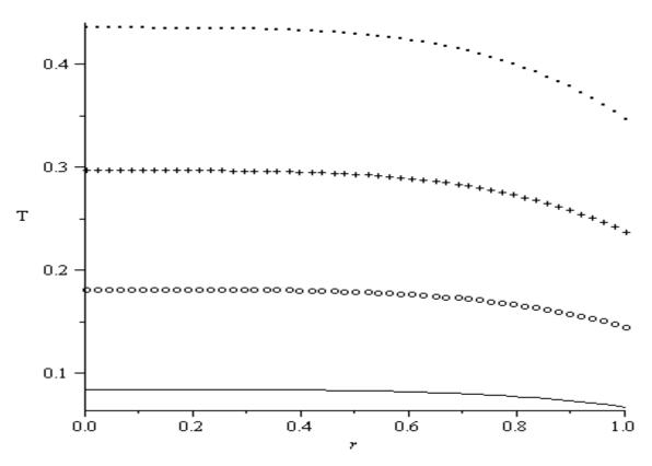
**Figure 8.** Temperature profile: G=1;  $\alpha = 1$ ; Bi = 1; \_\_\_\_\_Br = 1; oooooBr = 2; ++++ Br = 3; .....Br = 4.
