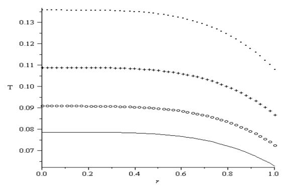
**Figure 6.** Temperature profile: G = 1; Br = 1; Bi = 1; a = 0.1; 00000 a = 2; ++++ a = 4; .....a = 6.
