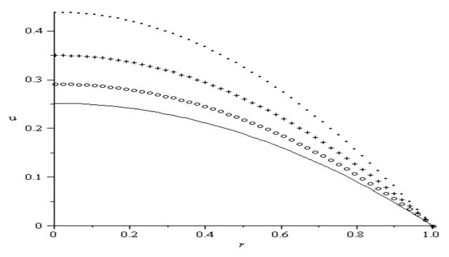
**Figure 2.** Velocity profile: G = 1; Br = 1; Bi = 1; a = 0.1; o = 0.1; o = 2;  $++++ \alpha = 4$ ; ..... $\alpha = 6$ .
