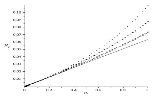
**Figure 13.** Total entropy generation: G = 1; Bi = 1; a = 0.1; o = 0.1; o = 0.2;  $++++ \alpha = 4$ ; ..... $\alpha = 6$ .
