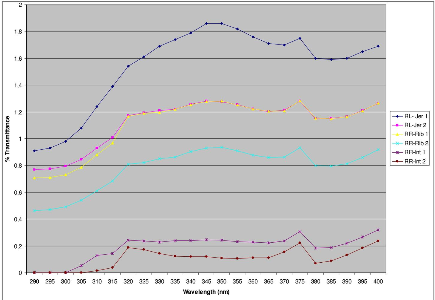
**Figure 4.** % transmittance values of 100% cotton knitted fabrics having dark color +4% UV absorbent substances of different constructions between 290-400 nm wavelengths.
