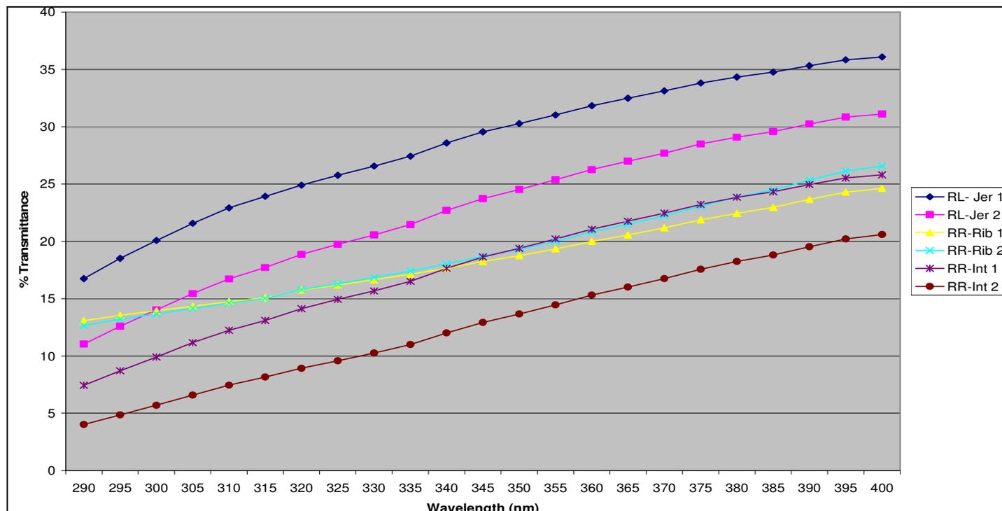
**Figure 2.** % transmittance values of knitted fabrics of different grams and constructions, on that applied hydrophilization process was applied, between 290-400 nm wavelengths.
