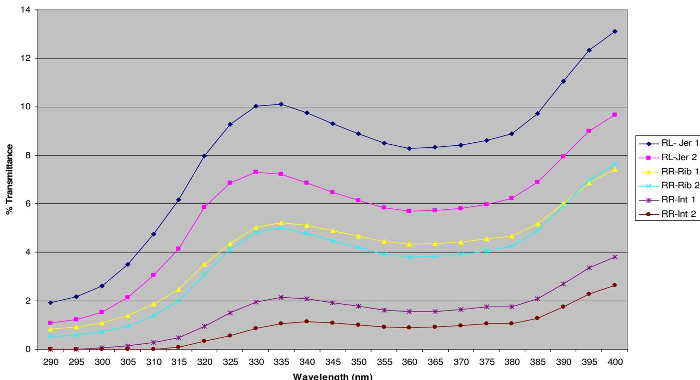
**Figure 3.** % transmittance values of 100% cotton knitted fabrics, which have optical bleach +4% UV absorbent substance and different constructions, between 290-400 nm wavelengths.
