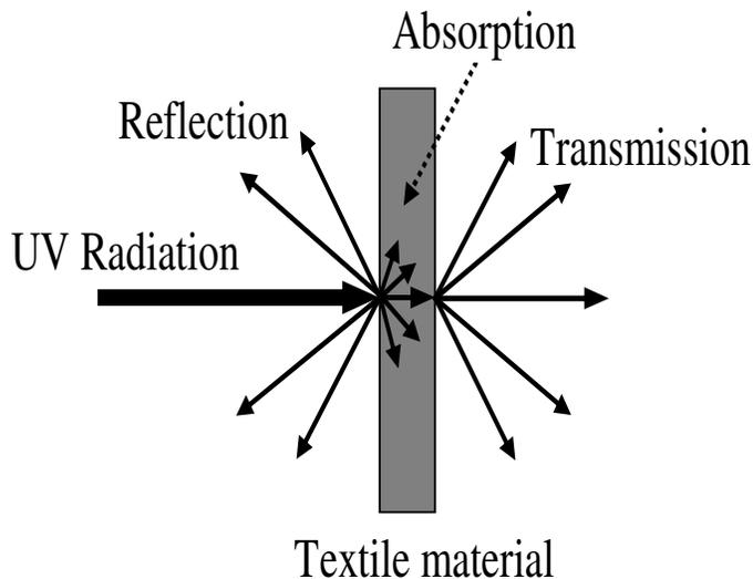
**Figure 1.** Reflection, absorption and transmission of UV radiation (Algaba and Riva, 2002).
