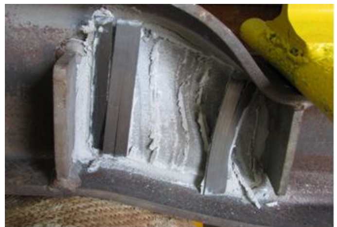
Figure 9c. Procedures of CFRP failing.
