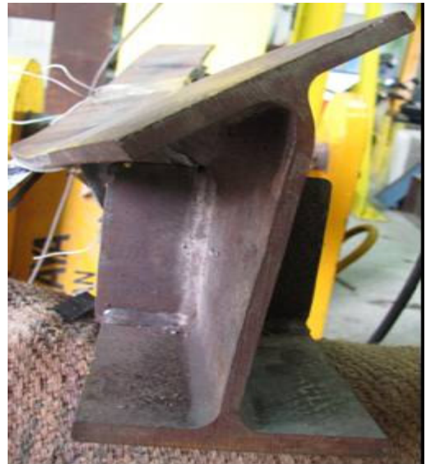
Figure 5a. Local yielding of web at the critical region.
