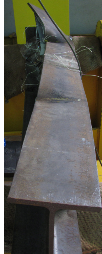
Figure 13a. Lateral-torsional-buckling (experiment).
