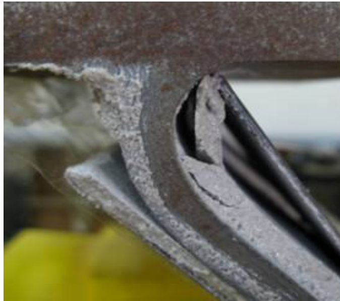
Figure 11. CFRP debonding on the tension and compression area.
