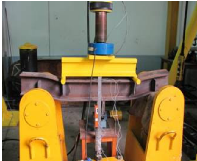
Figure 16. Vertical deflection of the specimen.
