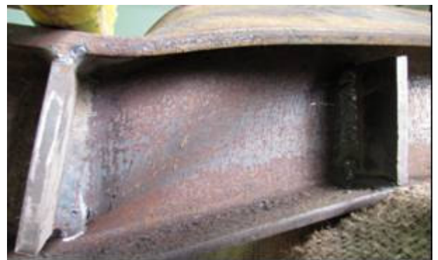
Figure 5b. Web crippling.
