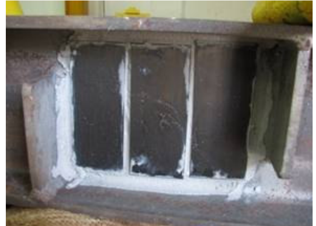
Figure 9a. Procedures of CFRP failing.
