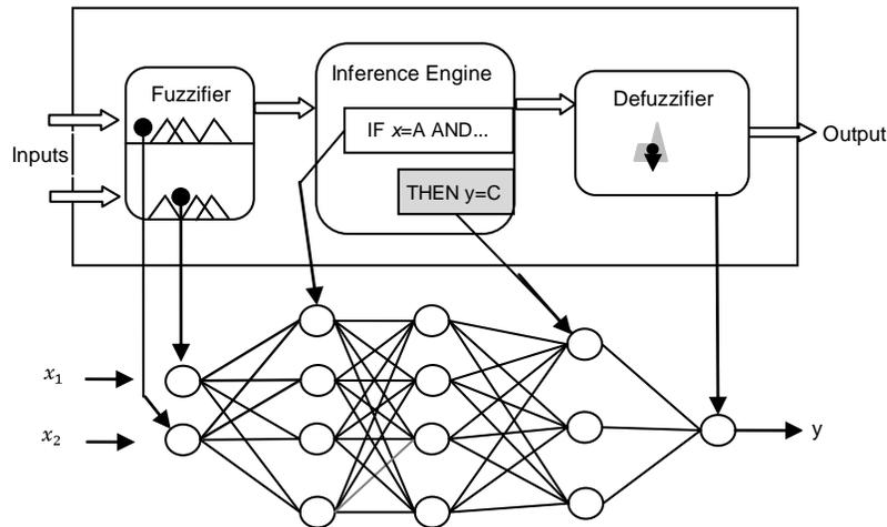
Figure 2. Structure of Hybrid N-F System (Ponnambalam et al., 2003).
