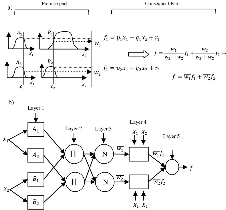
**Figure 3.** (a) Takagi-Sugeno fuzzy if-then rule and fuzzy reasoning mechanism; (b) equivalent ANFIS architecture (Aqil et al., 2007).
