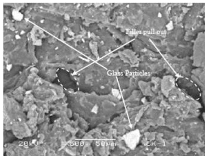
Figure 5. Worn surface of G1 specimen.
