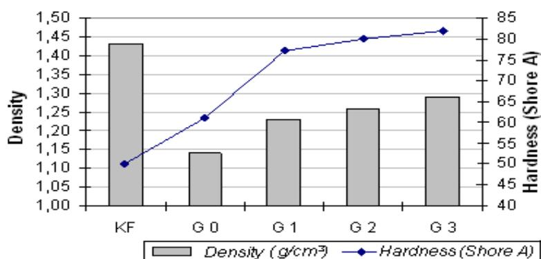
**Figure 1.** Changes in hardness and density values for classical and new formulae.
