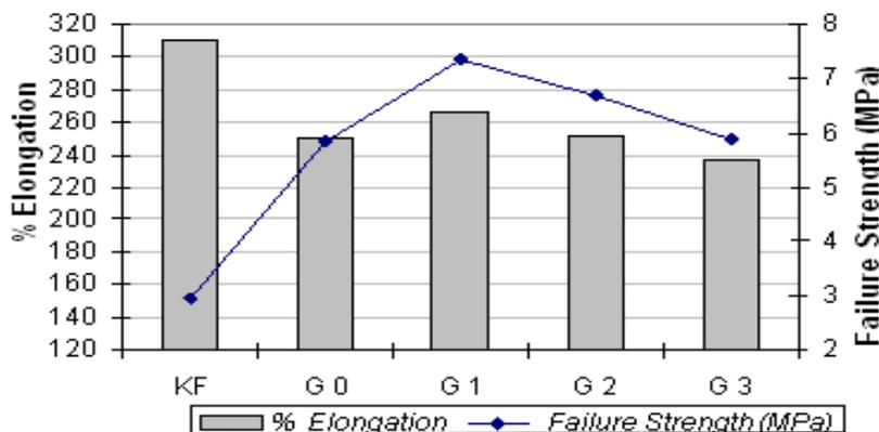
**Figure 2.** Elongation and failure strength in test parts for classical and new formulae.
