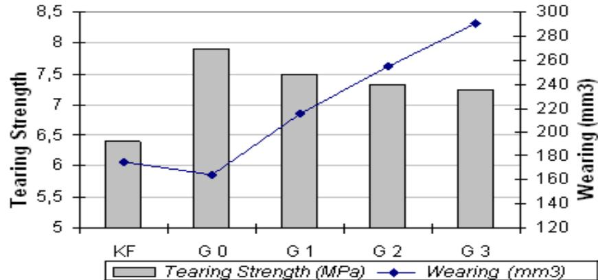
Figure 3. Changes in tearing strength and wearing amount for classical and new formulas.
