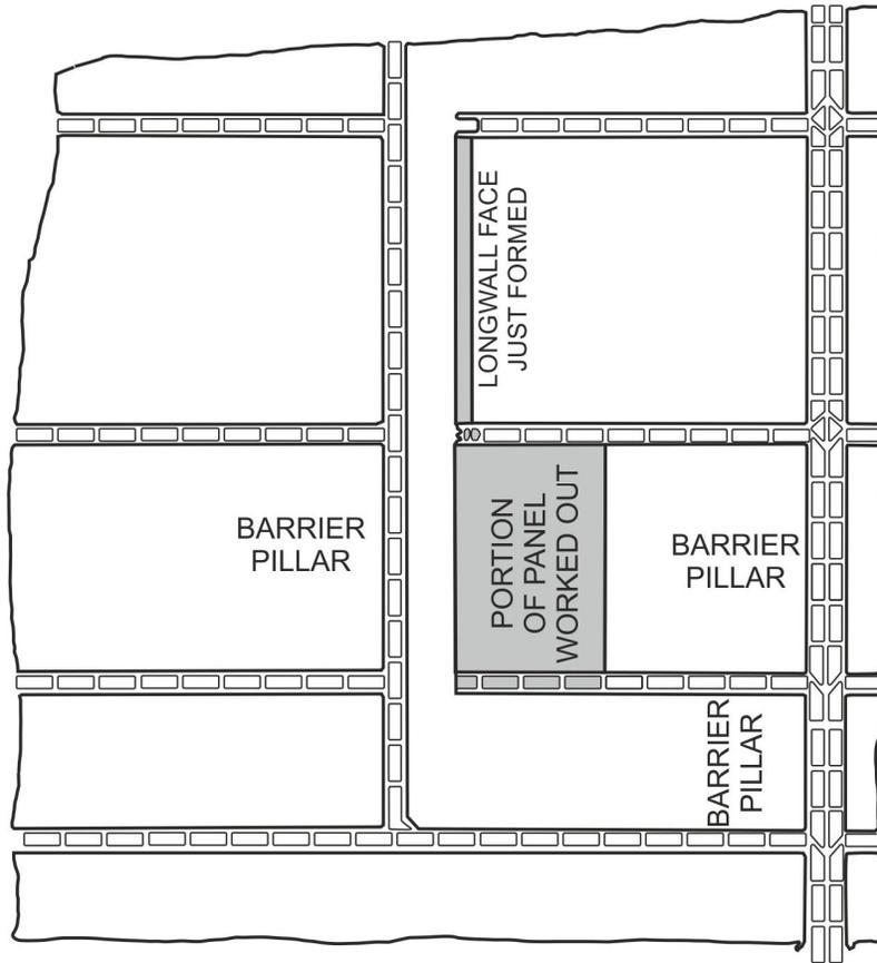
Figure 1. Longwall method in underground mining (Hamrin, 1980).
