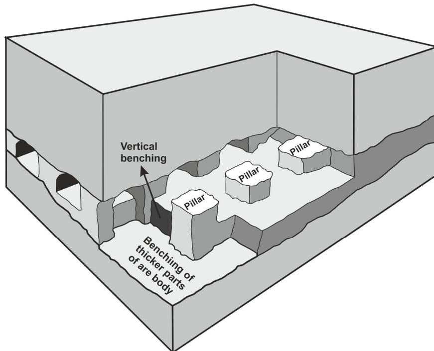
Figure 2. Room-and-pillar method in underground mining (Hamrin, 1980).
