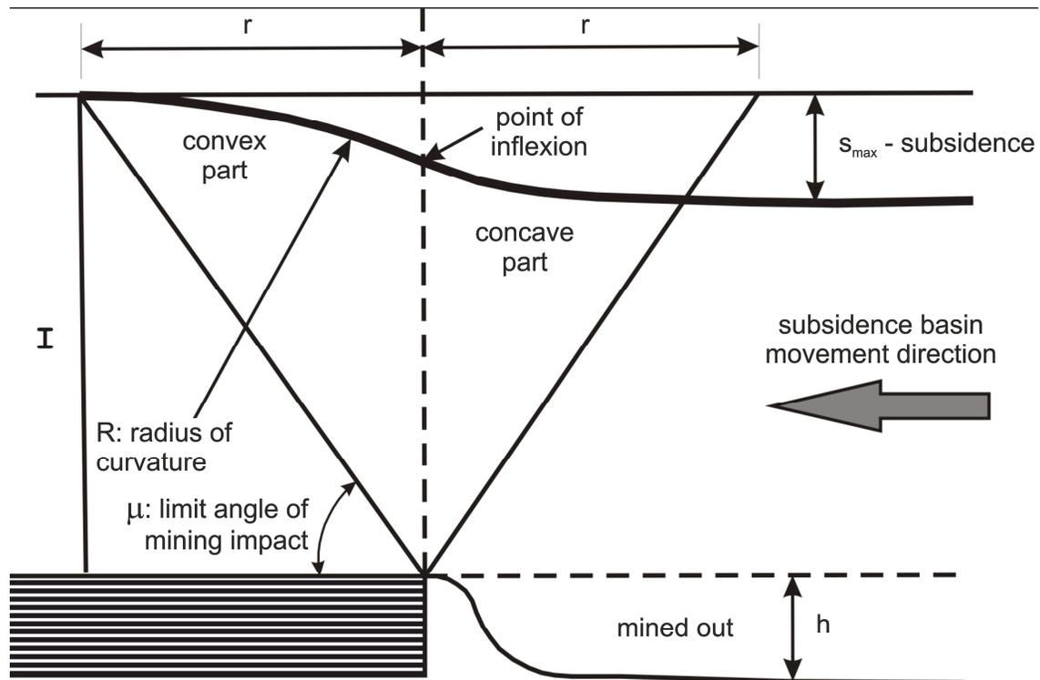
**Figure 3.** Schematic representation of influenced slope deformation by the subsidence (Marschalko et al., 2008; Marschalko and Treslin, 2009).
