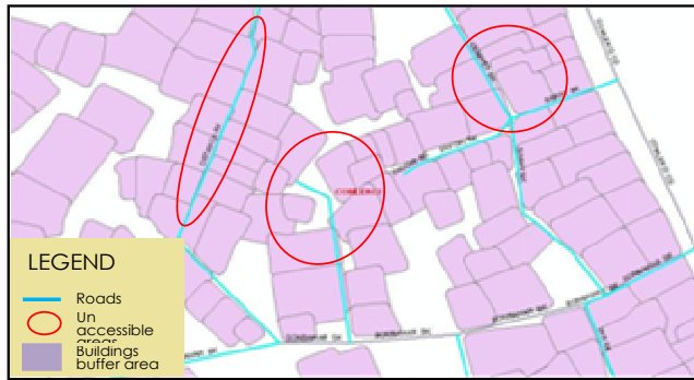
Figure 4. Sample for streets that a fire truck cannot enter (Cömlekci district, Ortanca and Cemiyet Street).
