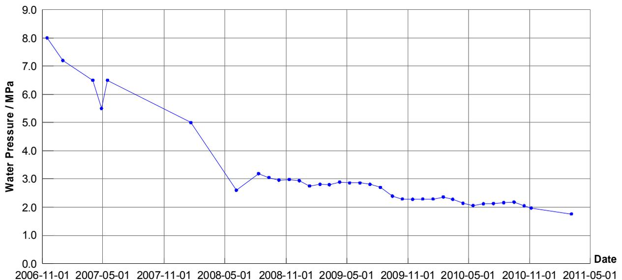
Figure 4. Water pressure of limestone corresponding to water drainage and pressure decrease.
