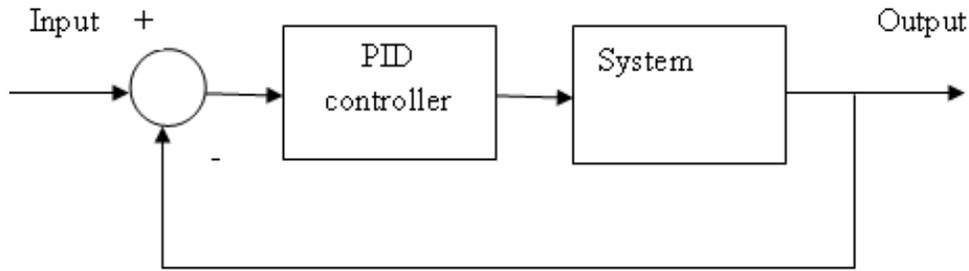
Figure 1. Block diagram for closed loop system.
