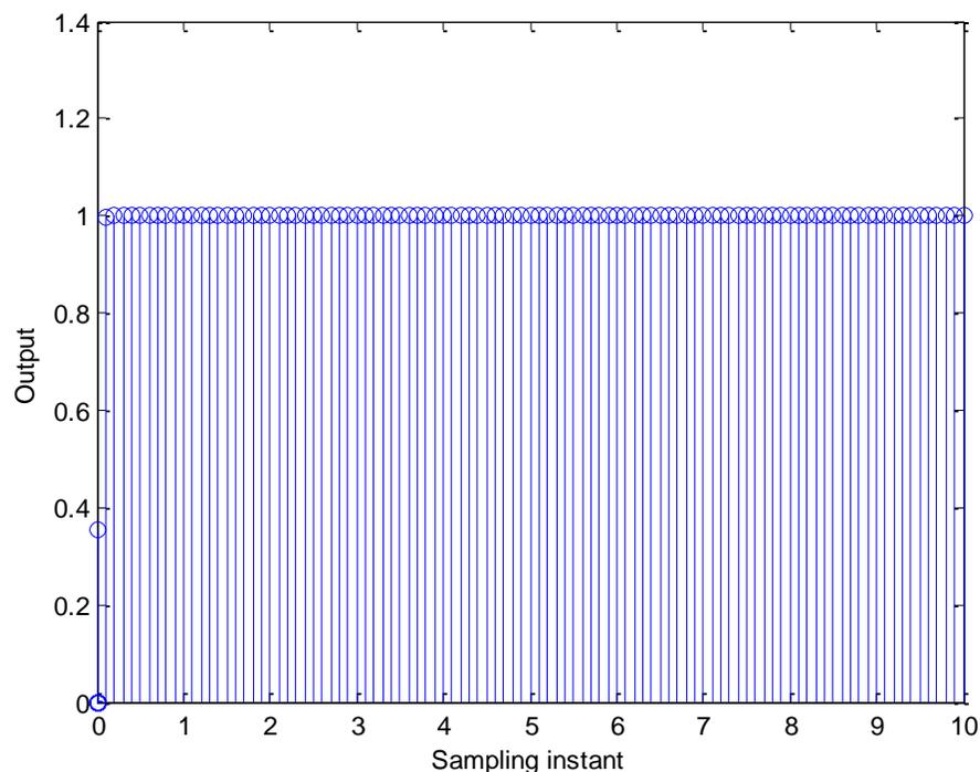
**Figure 6.** Step response of original system with PID controller of example 2.
