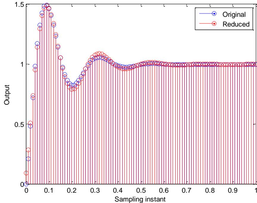
**Figure 2.** Comparison of step responses of original and reduced order system in example 1.
