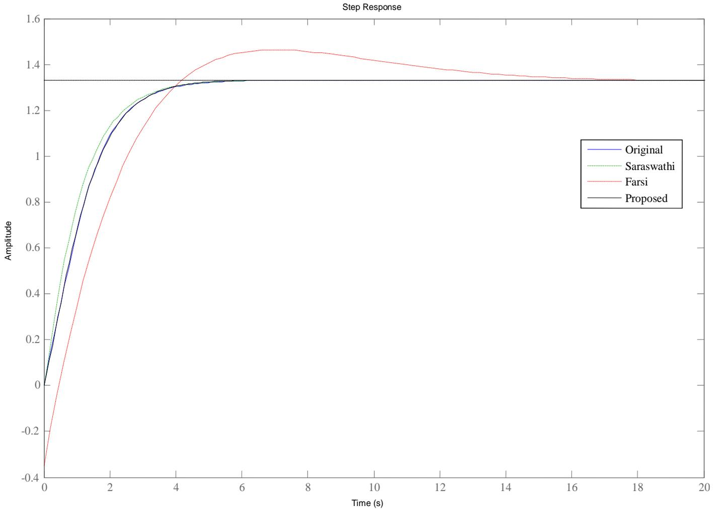
Figure 5. Comparison of step responses of original system and various reduced order systems of example 2.
