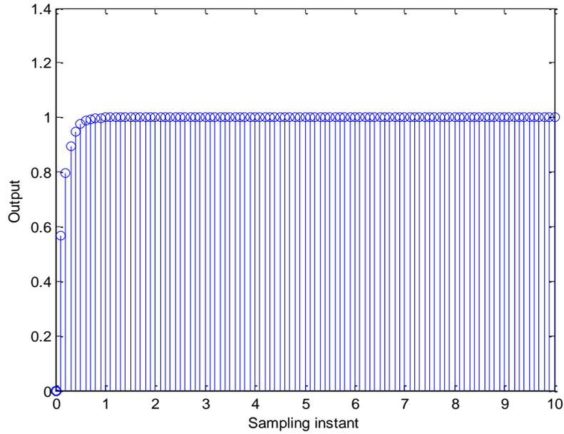
Figure 3. Step response of original system with PID controller of example 1.
