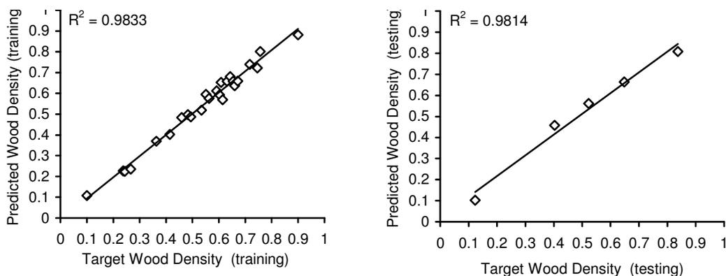
**Figure 3.** Relationship between the predicted and measured (target) values for wood density of *P. brutia* Ten. samples using FTIR spectroscopy via NN2 model.
