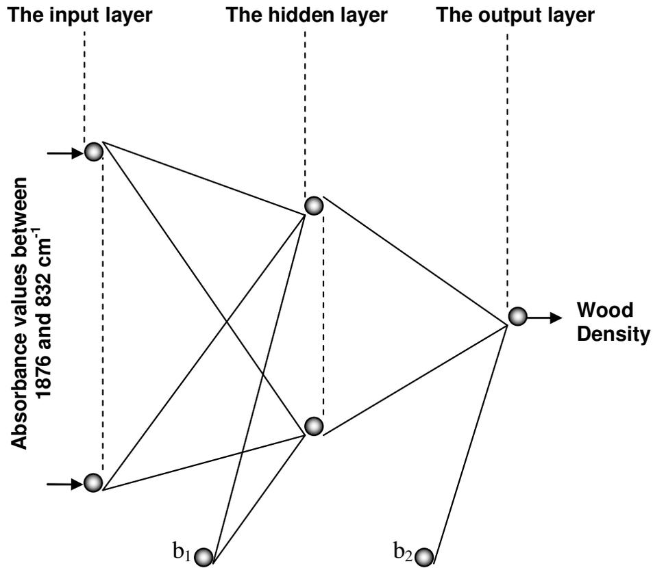
**Figure 1.** Network architecture used for prediction of wood density of *P. brutia* Ten. samples from FTIR spectral data.
