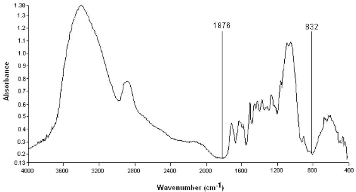
**Figure 2.** Typical FTIR spectrum of *P. brutia* Ten. wood sample.
