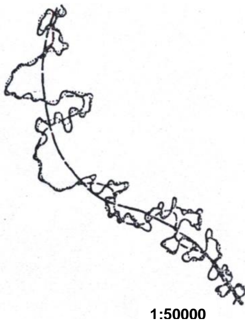
Figure 1. The actual and the general directions of the river flow of the certain size of the curve meandering for part of the river. On the map 1:50000 (VGI) curve meandering for the river Kolubara is given.
