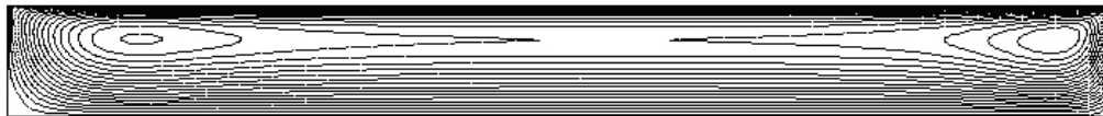
Figure 14. Contour of turbulent kinetic energy at Ri = 1 and for k - \varepsilon Standard turbulent model.
