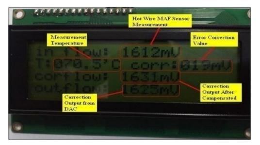
Figure 15. LCD Display for mass flow of 350 l/min.
