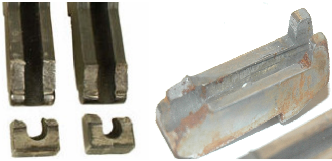
Figure 2. Fractured locking blocks.
